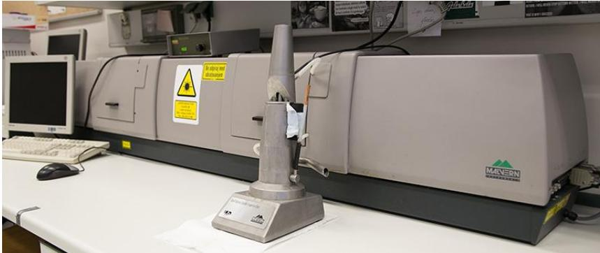
Device enables determination of particle size and size distribution of solid particles in size range between 0,05 and 900  $\mu\text{m}$  based on laser diffraction. The sample can be dispersed in air (i.e. using dry powder feeder and compressed air) or liquid (i.e. using small volume dispersion unit, the amount of liquid medium is  $\approx 100 \text{ ml}$ ).
