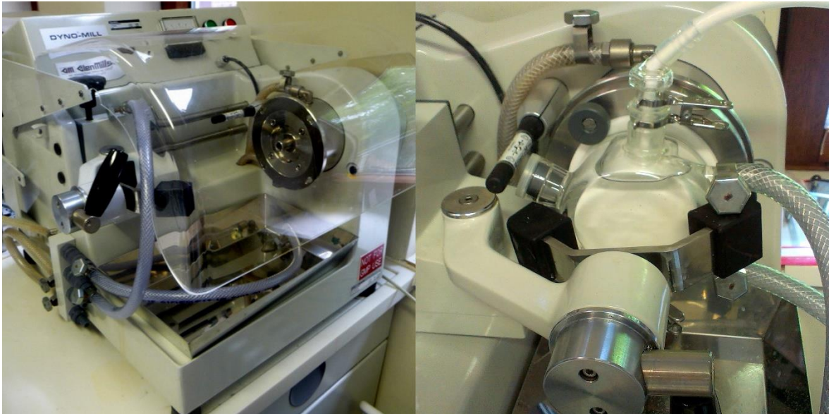
Figure 7: Left - Dyno Mill Typ KDL A, glassy milling chamber was adjusted to the stainless steel circle part just prior milling; right – glassy milling chamber with forced cooling water flow as a cooling system and pressure optimizer/releaser.
