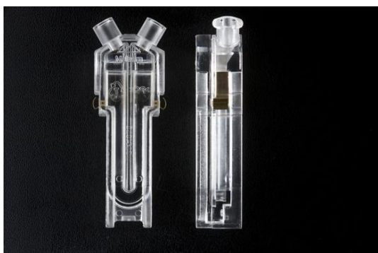
Figure 9: Disposable folded capillary cell. It has negative and positive electrode connected with a capillary, which is filled with a sample (40).
