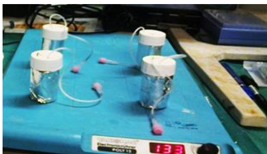
Picture 7: Dialysis with QuickSep system.
