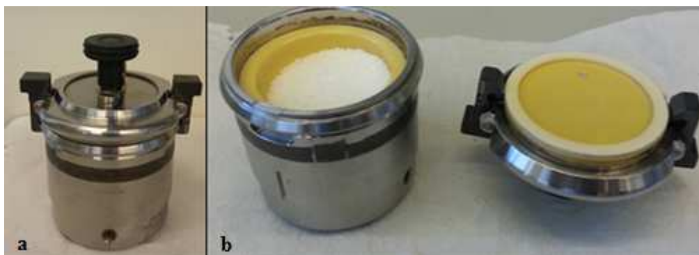
Figure 6: Grinding bowl: (a) closed and (b) opened and filled with milling pearls.
