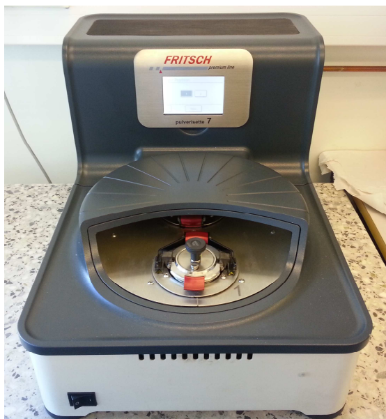
Figure 7: Planetary mill used for pearl milling in our research.
