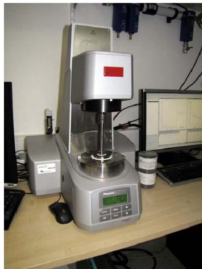
Slika 8: Reometer (Physica MCR-301) (28)
