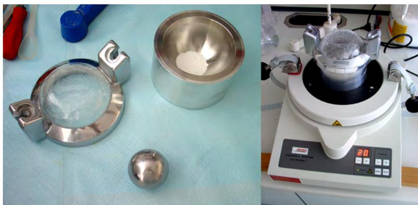
Fig. 13. Oscillatory ball mill Pulverisette 0.
