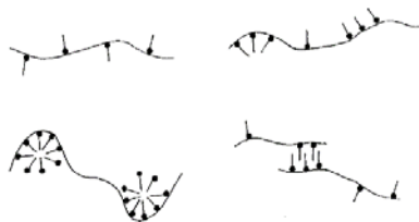
Fig. 7: Different bindings of polymer and surfactant molecules.
