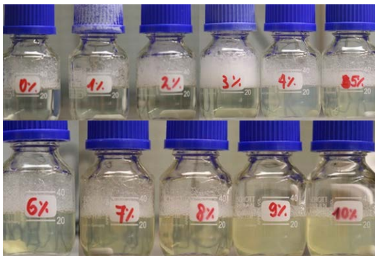
Fig. 10: Prepared solutions with pH 7 after stirring at 25°C. The % on the bottles indicates the amount of Na oleate in the solutions.
