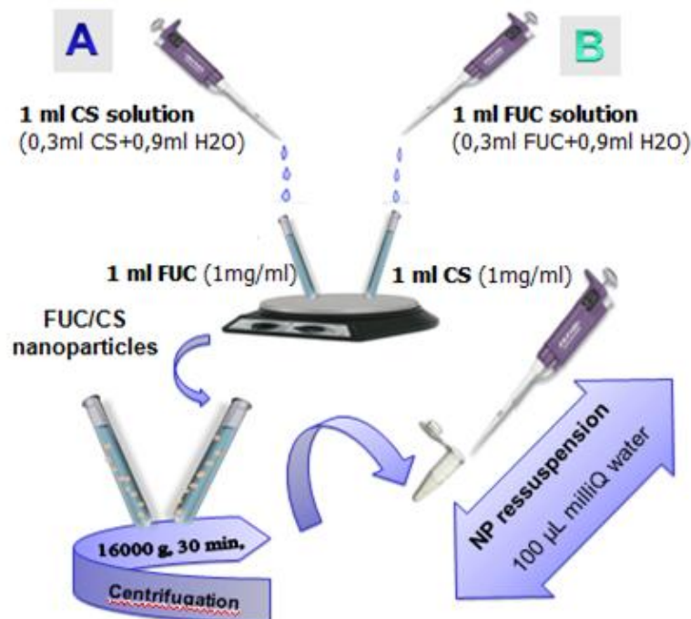
Figure 8: Preparation technique of the nanoparticles. Adapted from (23).
