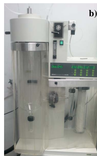
Figure 6: a) Büchi Inert Loop B-295; b) Büchi B-290 spray dryer (personal archive)
