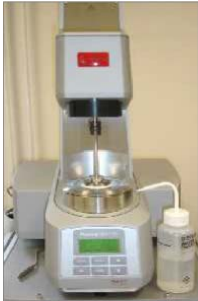
Slika 19: Reometer Anton Paar Physica MCR 301
