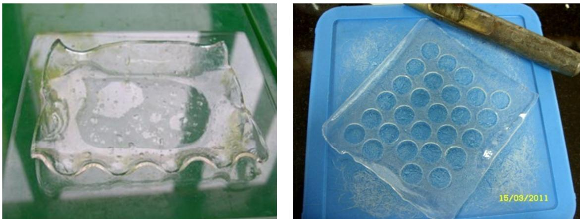
**Figure 12: Fully hydrated hydrogel sheet on the left and hydrogel sheet residue after lens cutting on the right.**
