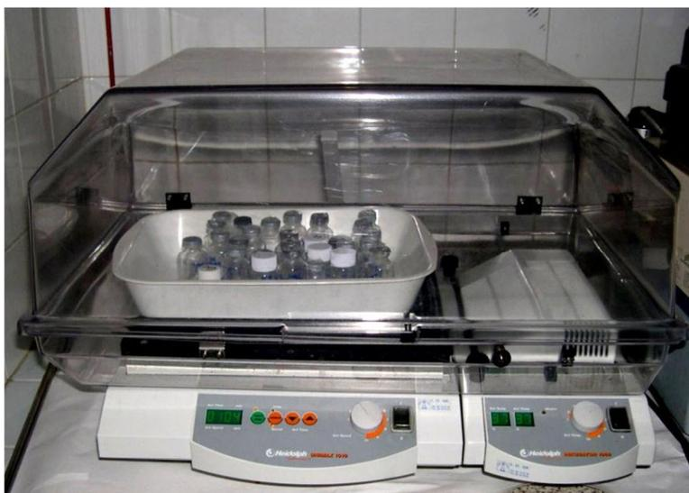
**Figure 10: The incubator platform shaker used for drug release.**
