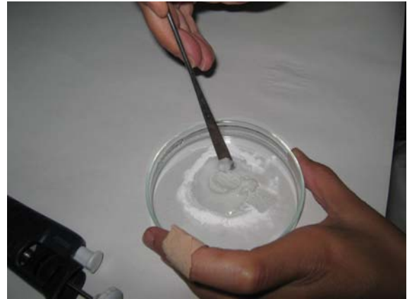
Figure 10. Homogenization of powder mixture (PMMA and lyophilised particles) with MMA with spatula in a Petri dish.
