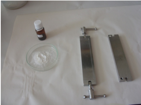
Figure 9. Material used in the preparation of acrylic bone cement. In the flask it is methyl methacrylate (MMA) and in the Petri dish it is polymethyl methacrylate (PMMA) with 10.0 mg of lyophilised particles. On the right side of the picture is the mould.
