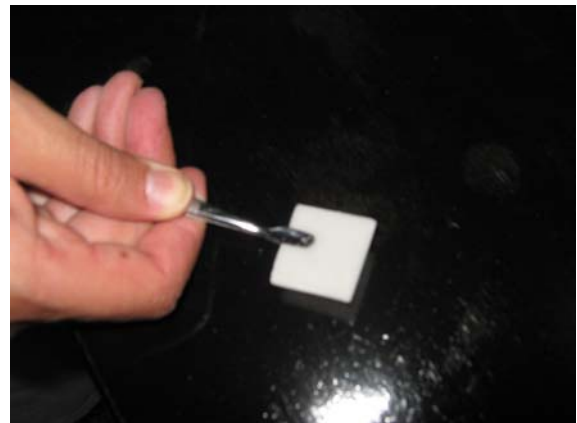
Figure 12. Plate of acrylic bone cement after completed polymerization.
