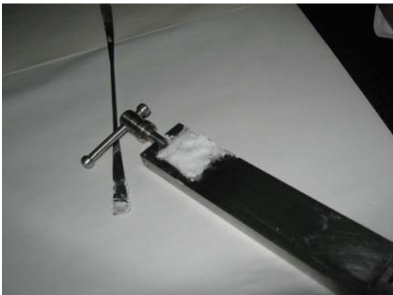
Figure 11. Acrylic bone cement mixture in the mould.
