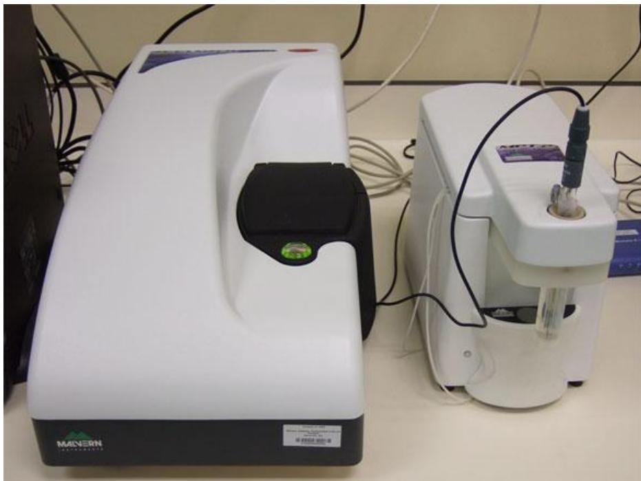
Photon correlation spectroscopy is the method for determination of particle size in the nanometric range (0.6 nm – 6  $\mu\text{m}$ ).
