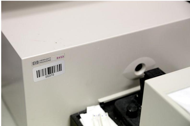
The instrument is used for qualitative and quantitative analysis of organic and inorganic substances by measuring their absorbance in the solution at different wavelengths.
