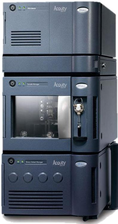
The latest generation of HPLC instruments, that can generate pressures to 1000 bar.
