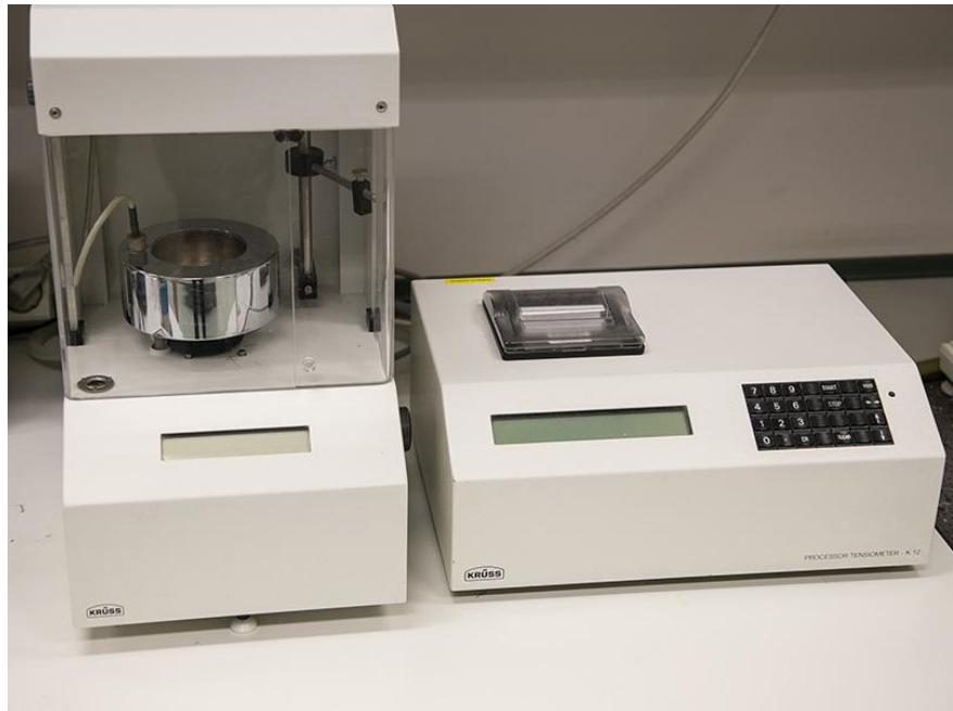
**Tensiometer K12 is used for reliable measurements of surface tension and interfacial tension.**
