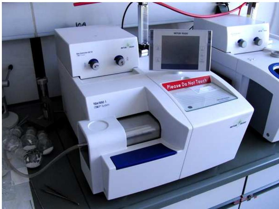
Thermogravimetric analysis (TGA) describes any experimental method whereby changes in mass are used to detect and to measure the chemical and, less frequently physical processes that occur on heating a sample under investigation.
