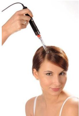
**The instrument is used to measure the pH on the skin surface or on the scalp.**
