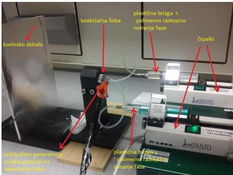
**Device for electrospinning enables the formulation of single or coaxial nanofibers from different solutions of synthetic or natural polymers.**
