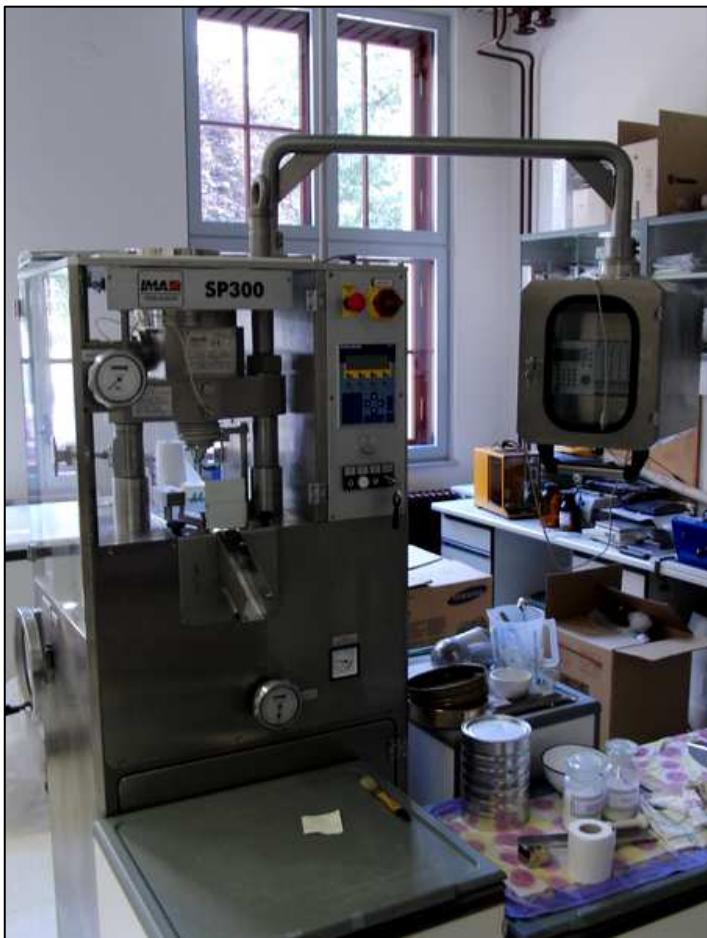
Single-punch tabletting press SP300 is fully instrumented machine and enables measurements of upper and lower punch forces, ejection force and displacement of the upper punch. It is well suited for advanced studies of compressibility, as well as analysis of force-displacement curves. It is equipped with gravity and forced filling shoes. The machine has a wide spectrum of applicability from manual production of only a few tablets to batch production on semi-industrial scale.
