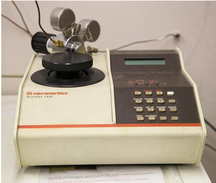
**By He-pycnometer the true density of solids can be determined.**
