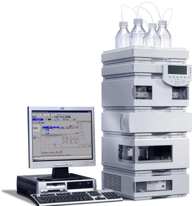
The instrument enables chromatographic detection and quantification of substances, API's, their degradation products and metabolites.
