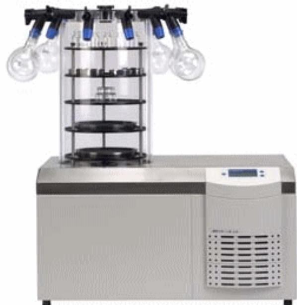
**Freeze drying is the process by which water is removed from a frozen material by sublimation. It is used for drying delicate, heat-sensitive materials of high value or to achieve a porous structure.**
