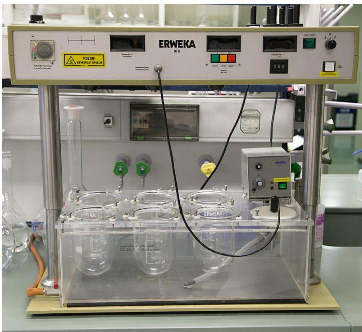
Erweka DT6 dissolution test device can be used as Basket Apparatus (Apparatus 1) or Paddle Apparatus (Apparatus 2).
