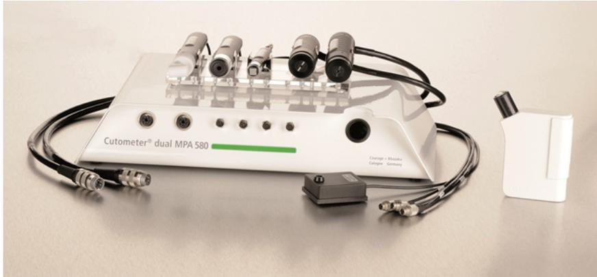
The instrument is used to determine biomechanical parameters of the skin (firmness, elasticity).
