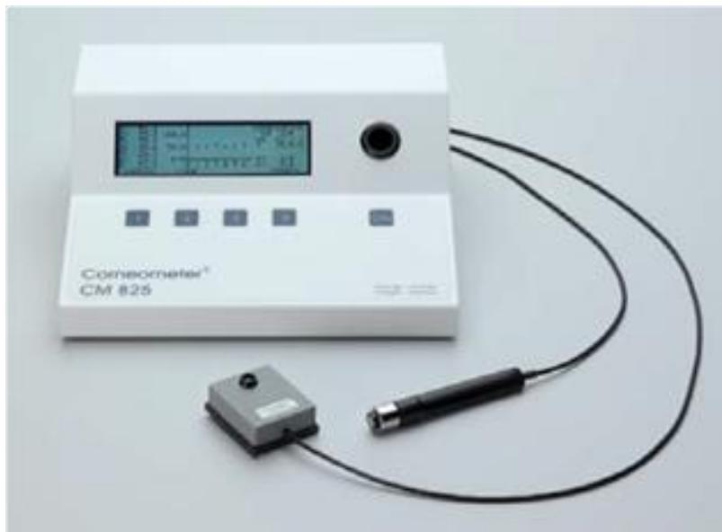
The instrument is used to determine the skin hydration (water content in the stratum corneum).
