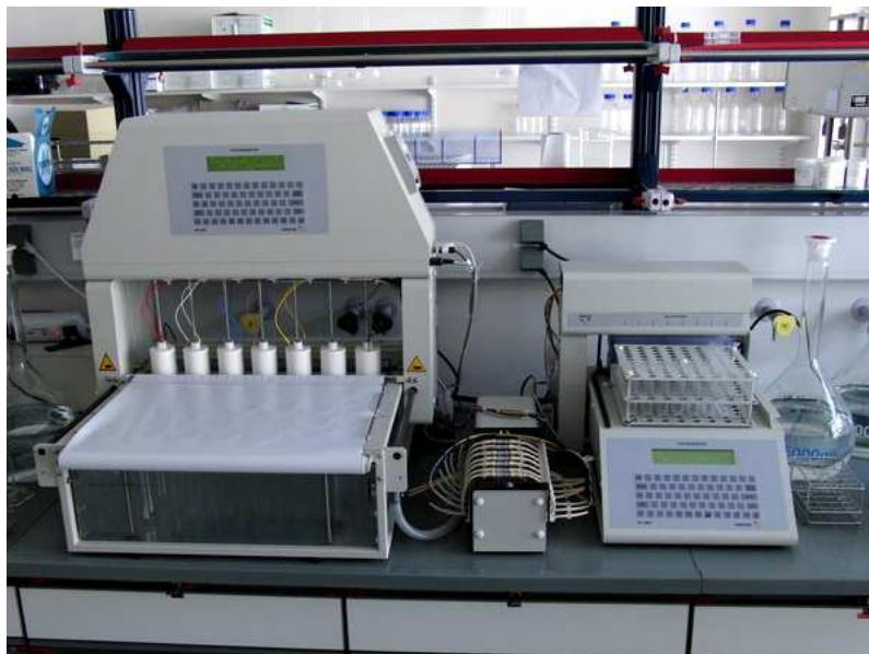
BioDis apparatus enables observation of drug release from oral dosage forms with modified release: delayed, prolonged, pulsative. The apparatus is accompanied by auto-sampler.
