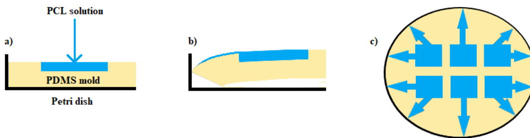
Fig. 15: a) Petri dish side view: PCL solution poured in the PDMS mold, b) swollen PDMS mold with PCL solution flowing over the edges of PDMS mold, c) Petri dish top-view: PCL solution flowing over the edges of PDMS mold in different directions.
