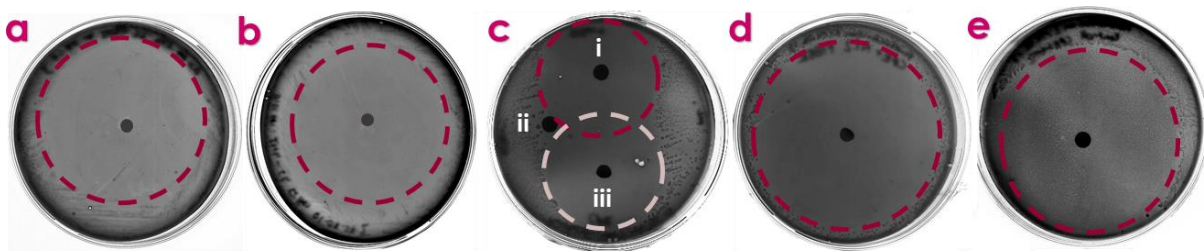
Figure 31: Inhibition zones of a) metronidazole nanofibers, b) metronidazole positive control, c) i: ciprofloxacin nanofibers, ii: filter paper, iii: ciprofloxacin positive control, d) nanofibers with combination of drugs and e) metronidazole + ciprofloxacin positive control on F. nucleatum .
