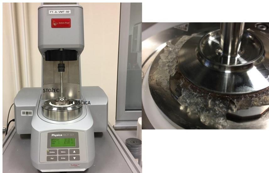
*Slika 14: Reometer Anton Paar Physica MCR 301 s senzorskim sistemom CP50-2.*
