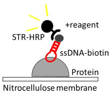
**Figure 3.4: The scheme of ECL visualization.**
