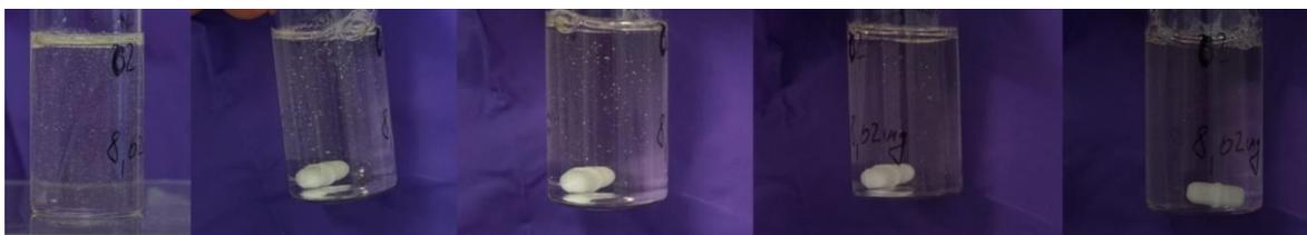
Figure 17: C2 sample - from left to right: 0, 1, 3, 5 and 21 hours of magnetic stirring at 4 °C.
